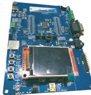
1 | GD32150R-EVAL Evaluation kit for the GD32 ® Cortex ® -M3 GD32150R8T6 MCU
